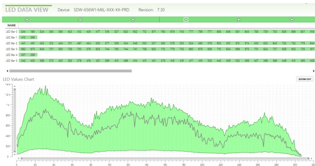
Figure 3: Graph representing LED values while on baseline testing (0 dead LEDs)
