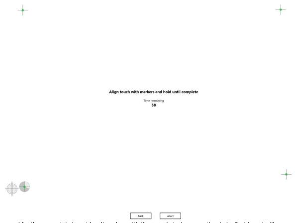
Note: It is normal for the green dots to not be aligned up with the cross hair shown on the circle, Dashboard will measure this offset and use it to calibrate the screen.
